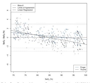
This graph shows plots of the error  $(SpO_2 - SaO_2)$  by SaO<sub>2</sub> using the 3230 with a linear regression fit and upper 95% and lower 95% limits of agreement. Each sample data point is identified by subject from a clinical study in non-motion conditions.
